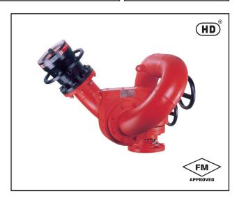
The monitor has welded carbon steel 6 inch (150 NB) water way. All steel parts are hot dip galvanized and epoxy painted for excellent corrosion resistance. The vertical and horizontal rotation is through corrosion resistant bronze swiveling joints with double row of stainless steel ball bearing. Both vertical and horizontal movements are controlled with handwheel driven fully enclosed worm gears and protected from the elements.
