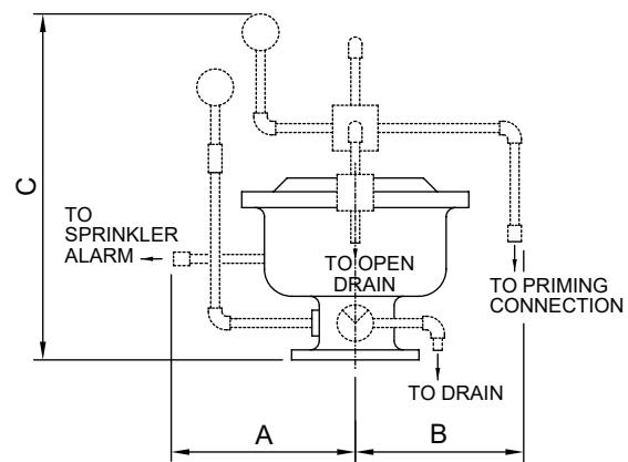
**INSTALLATION MEASUREMENT IN MM
