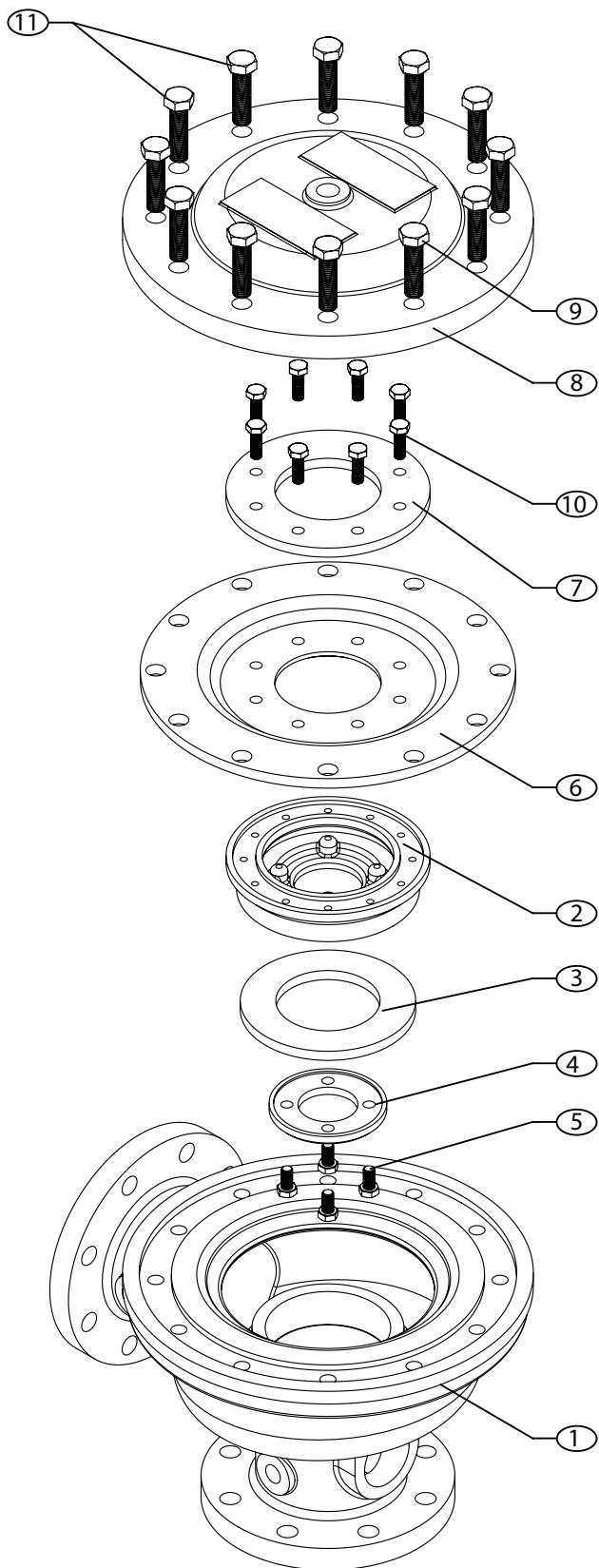
**DRY PILOT BASIC TRIM ASSEMBLY FOR DELUGE VALVE MODEL - A WITH TEST & ALARM, DRIP & DRAIN VALVES, SIZES - 50/80/100/150 & 200NB - NTD**
