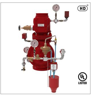
When fire is detected through wet pilot sprinkler system, the primary water control deluge valve opens, allowing water flow into the sprinkler piping in readiness for possible subsequent opening of one or more sprinklers.
