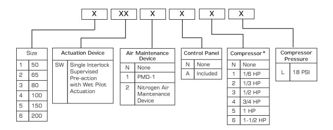
\*Compressor standard supply is 50 Hz., 60 Hz is optional supply.
