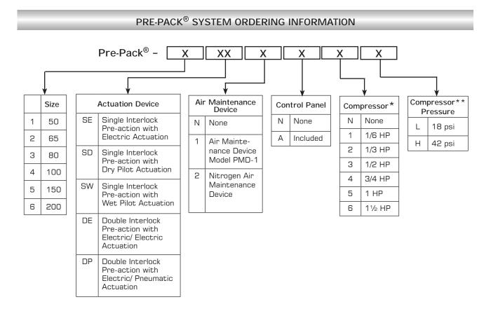
\*Compressor standard supply is 50 Hz., 60 Hz is optional supply. Installer to specify the compressor capacity required depending on pipeline volume.
