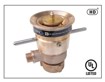
The debris trapped in the nozzle may effect the nozzle performance. To remove trapped debris, the water flow must be stopped and thereafter carefully unscrew and remove the nozzle deflector. Clean the nozzle and reassemble. While reassembling the nozzle or as a normal preventive maintenance, water proof lubricant must be used on seal and moving parts for smooth operation. The nozzle must be operated periodically under full flow jet as well as under fog pattern.
