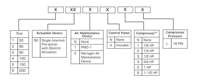
\*Compressor standard supply is 50 Hz., 60 Hz is optional supply.
