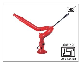
The monitor has welded carbon steel water way. All steel parts are hot dip galvanized and painted for excellent corrosion resistance. The vertical and horizontal rotation is through corrosion resistant bronze swiveling joint with double row of stainless steel ball bearing. Both vertical and horizontal movements are controlled with handle with twist lock.
